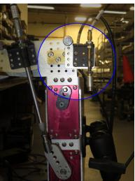
8. Reconnect the corresponding cable's quick disconnect to the servo arm.
