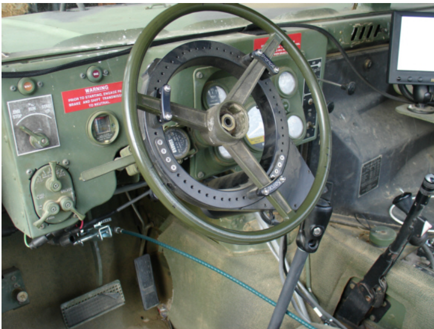
Steering Ring installed in a military HMMWV.
