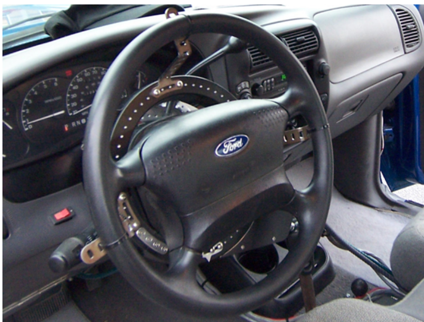
Steering Ring installed in a Ford Ranger.
