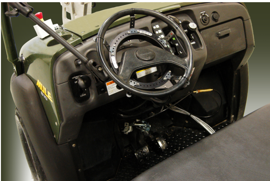
Steering Ring installed in a Kawasaki Mule.
