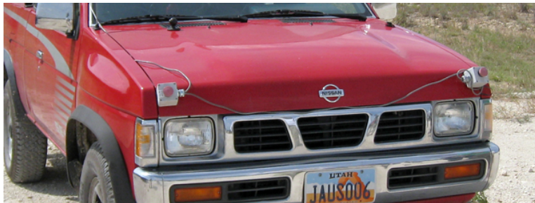
Figure 3: Hardwired E-stop buttons place on the exterior of an unmanned vehicle
