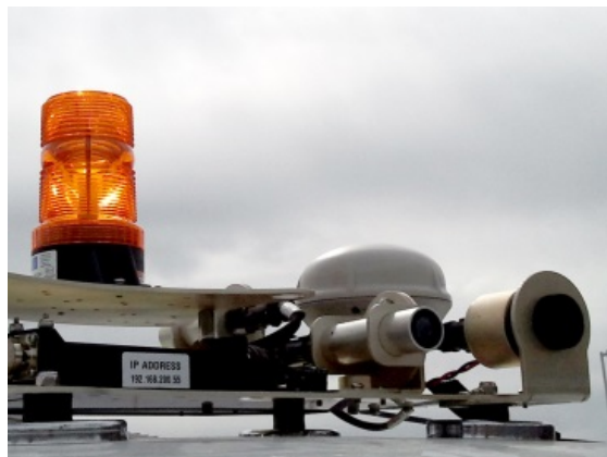
Figure 2: Warning Light and Audible Alarm
